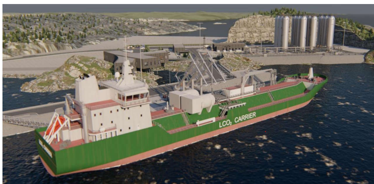
Figure 2: LCO2 Vessel (7500cbm 3 ).
